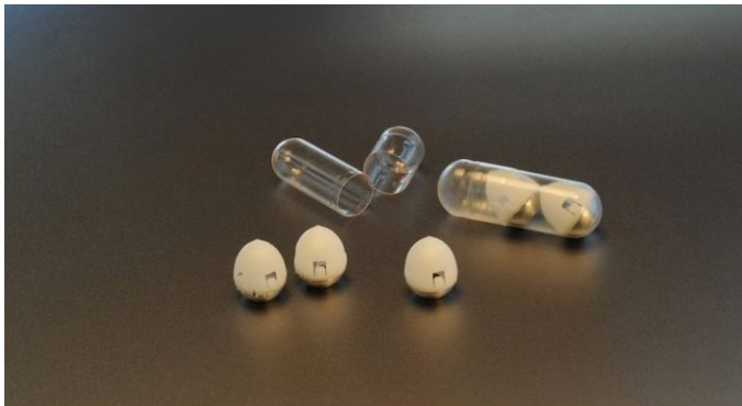
Fig. 2 The SOMA self-oriets quickly from any position and remains stable once oriented.
